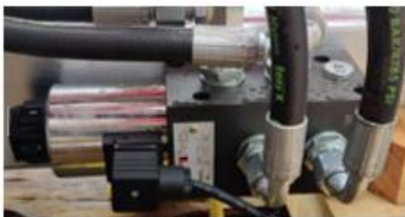
6 Port Solenoid valve, Part Number MS001106
