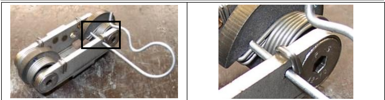
Fig. 12: Tensioning the excentric with a clip
