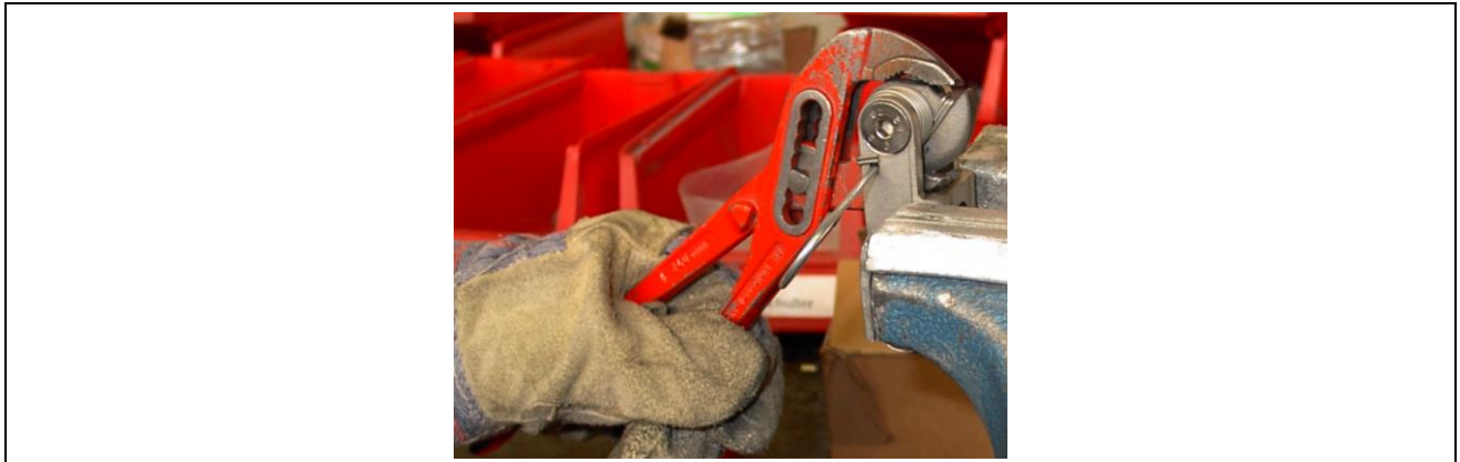
Fig. 13: Tensioning the excentric with water pump pliers
