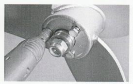
Loosen 3x V2A-M12-hexagon screws (WAF19). Remove the screws and limes rings (conical lock washer).
