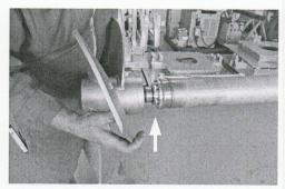
3. Slip the new propeller on the tube. Take care, 4. that the bearing housing flange and agitator shaft have little erosion, otherwise replace the bearing housing and if necessary use SUMA-protective tube.
