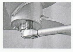
(WAF19) with limes rings and tighten them with 70 Nm.
